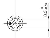
Groove for parallel key A5x3x28 to DIN 6885 T3
