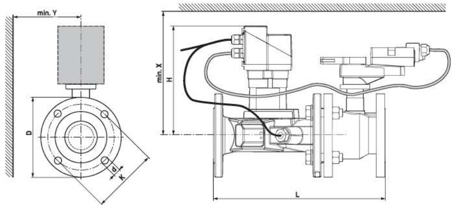
If Y < 180 mm, the extension of the hand crank must be demounted as necessary.
