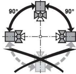
**Installation position in return** Installation in the return is recommended.
