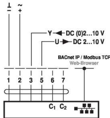
Override control and limiting with DC 24 V with relay contacts (with conventional control or hybrid mode)
