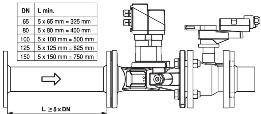
**Mounting of immersion sleeve and temperature sensor**
