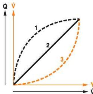
**Power control** Alternatively, the control signal DDC can be assigned to the output power required at the heat exchanger.
