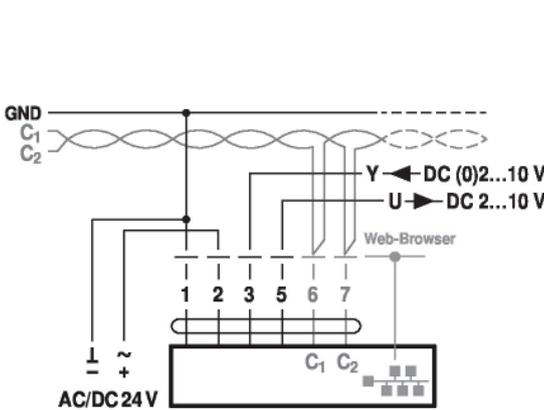
BACnet IP / Modbus TCP with analog setpoint (hybrid mode)
