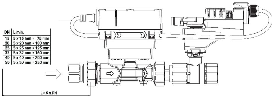
**Split installation** The valve-actuator combination may be mounted separately from the flow sensor. The direction of flow of both components must be observed.
