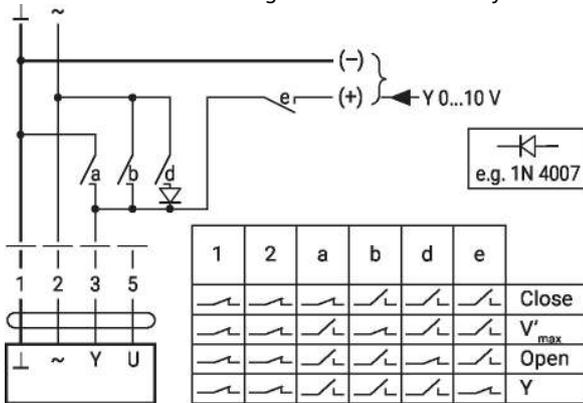
Override control and limiting with DC 24 V with relay contacts (with conventional control or hybrid mode)
