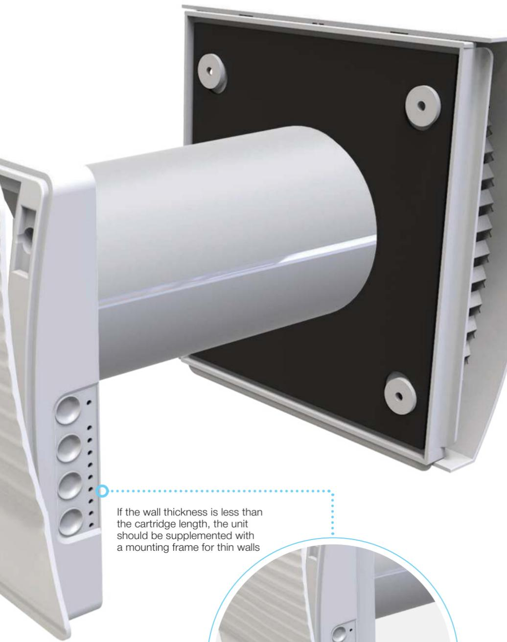
If the wall thickness is less than the cartridge length, the unit should be supplemented with a mounting frame for thin walls
