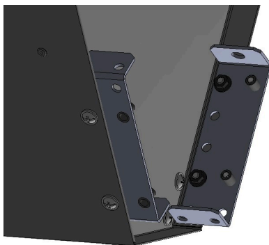
Installation of connector inside the curtain
