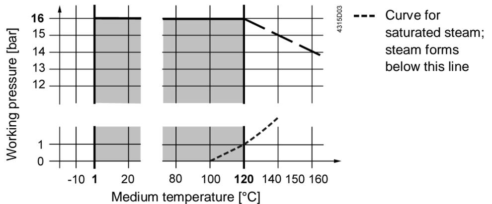
**Working pressure and medium temperature staged as per ISO 7005**
