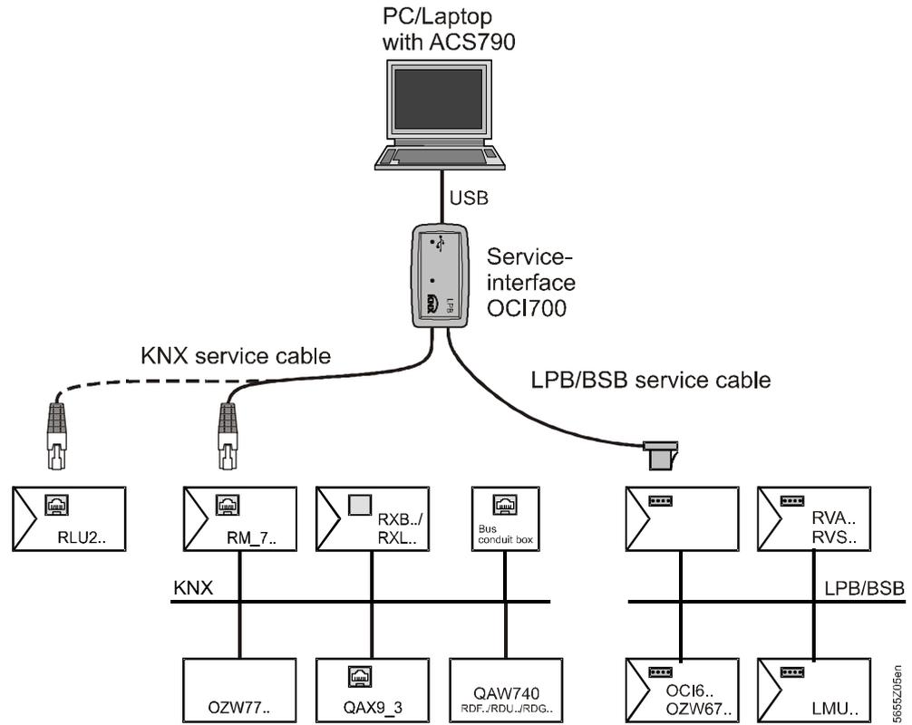
Select connection In ACS790, select the associated connection to communicate with the devices, i.e. "OCI700-KNX" or "OCI700-LPB".
