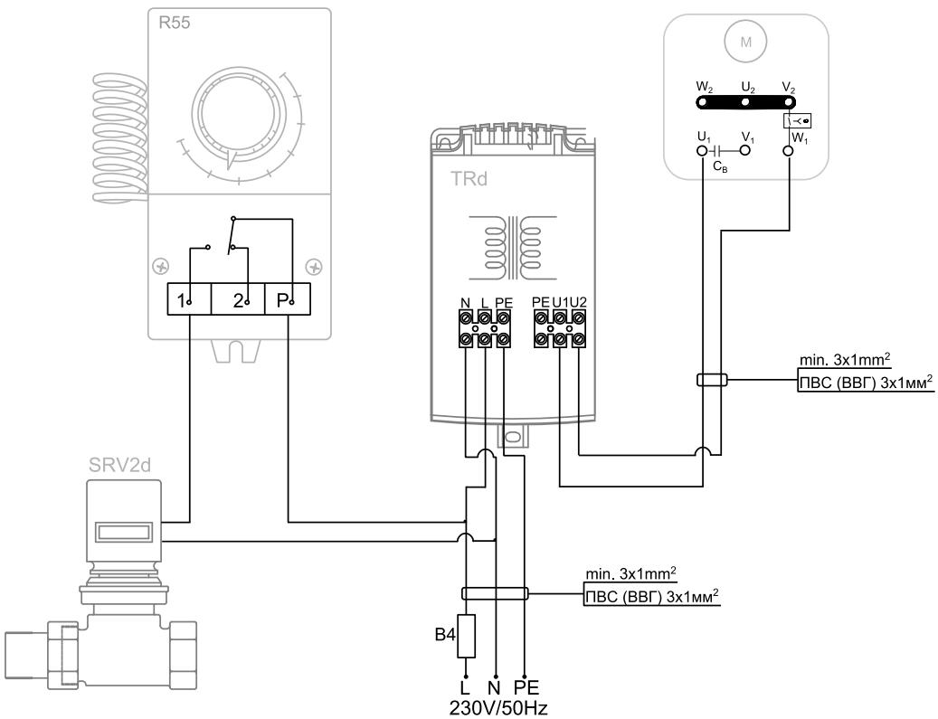
Thermostat R55 controls the operation of SRV2d valve. TRd speed regulator allows for 5-step fan air flow switch.
