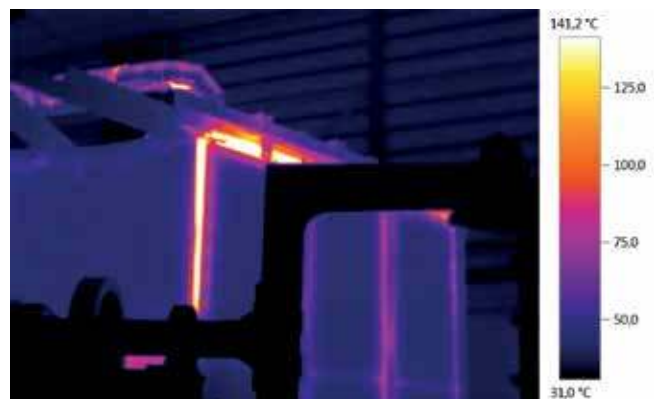
Industrial kiln with faulty insulation.
