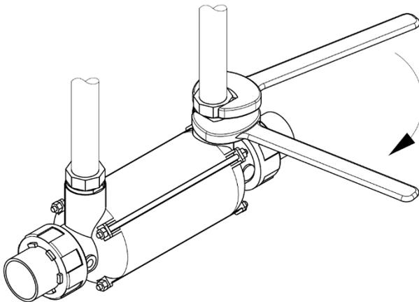
To prevent the stainless-steel fitting from detaching itself from the heat exchanger housing and, as a result, also from the corrugated coil, and to prevent leaks from occurring, the stainless-steel fitting should be firmly tightened with a second spanner or pliers.
