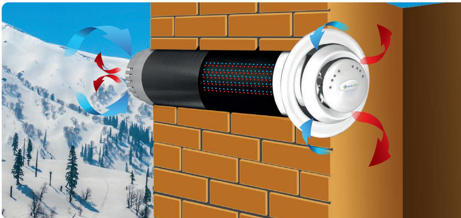
The air flows are not mixed, but move in different channels of the heat exchanger. Due to this, the temperature is transferred from the exhaust air to the supply (recuperation). Due to this, the energy efficiency of recovery is up to 93%.
