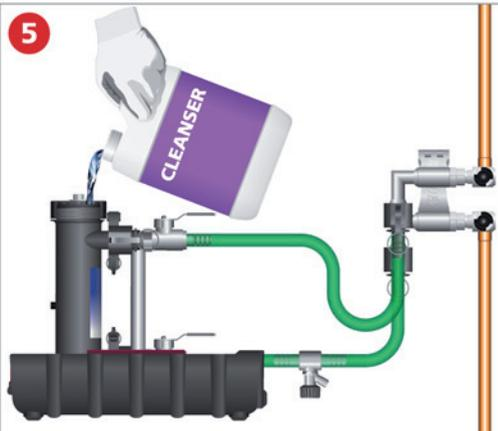
Add recommended cleanser to the system via the *RapidFlush Filter* canister.
