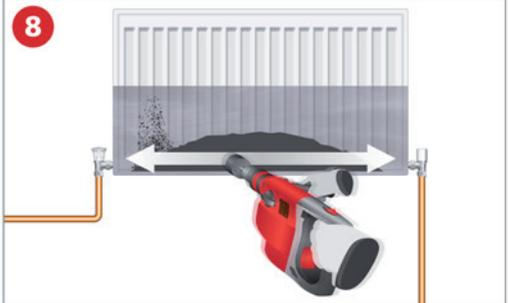
Turn off any by-pass valves and all the radiators, leaving only one radiator open at a time. With the system running, agitate each radiator using ADEY's *VibraClean* tool attached to an SDS drill for 15–20 seconds.
