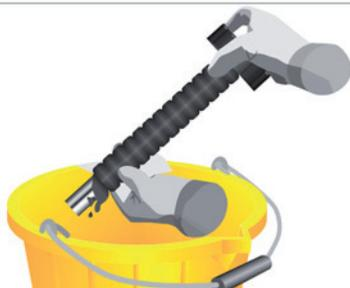
Isolate and clean the *RapidFlush Filter* as required. Using Personal Protective Equipment i.e. gloves and paper towels, wipe off any magnetite into a bucket or waste bag and dispose of correctly. When satisfied, open up the next radiator, turn off the treated radiator and repeat the process until all radiators are clean.
