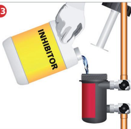
Add a recommended inhibitor into the canister i.e. use the Pro-Fill bleed valve or remove canister lid assembly and pour into the filter (holds approximately half a litre). Open up the isolation valves and remove any air.
